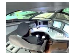
Conduct test run for driverless Shinkansen operation (GOA4)
