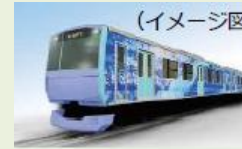
Development of test railcar for hybrid railcar (fuel cell) that uses hydrogen as energy source
