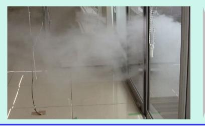
[Positive pressure-controlled store: Equal pressure inside and outside of store]  $\rightarrow$  Outside air does not flow into store
