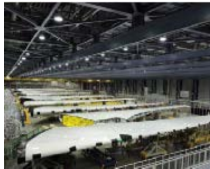
787 main wing assembly line
