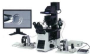
**The ICSI system is based on the Olympus IX3-SLICSI inverted microscope**
