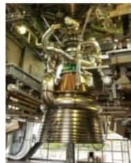
Preparation of combustion testing of 1st-stage engine
