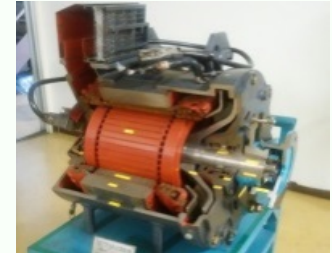
Cut model of railcar electric motor
