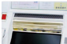
Mirror Allows the ATM user to view the situation behind them
