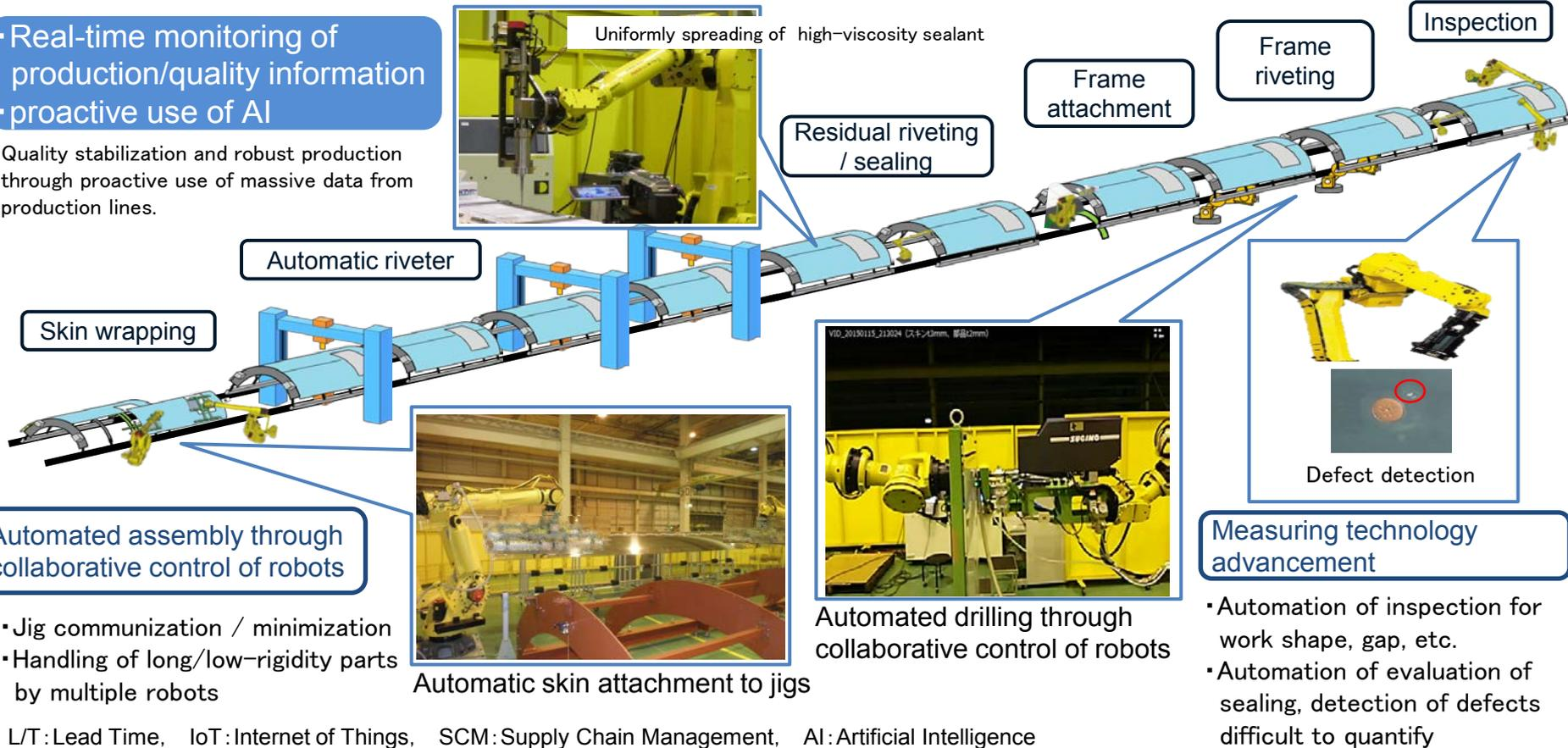
Automated assembly through collaborative control of robots
