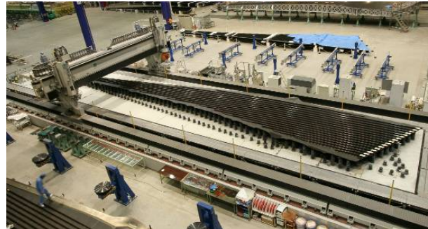
Water-jet cutting machine for skin (Expanded)
