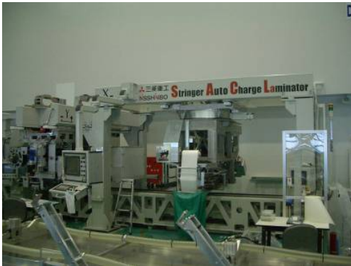
Automatic laminator for stringers (Expanded)
