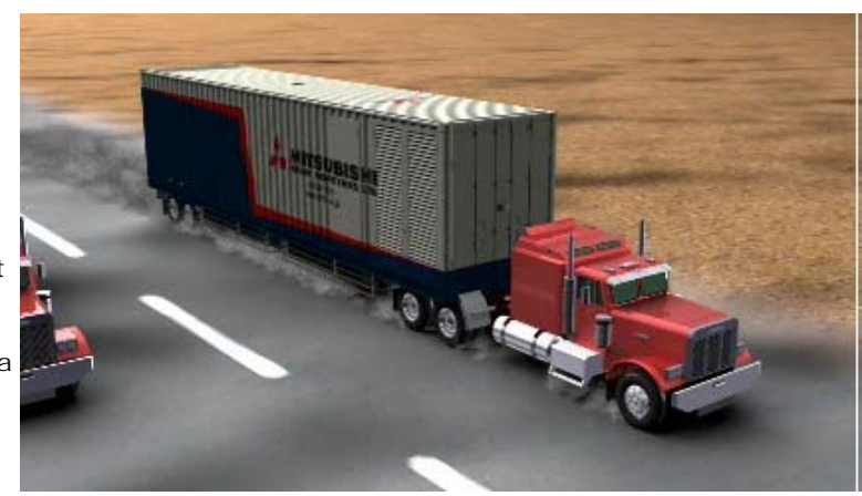
A container-type gas power generation system: As its installation is finished just by placing it, it can be put into operation in a day at the shortest.
